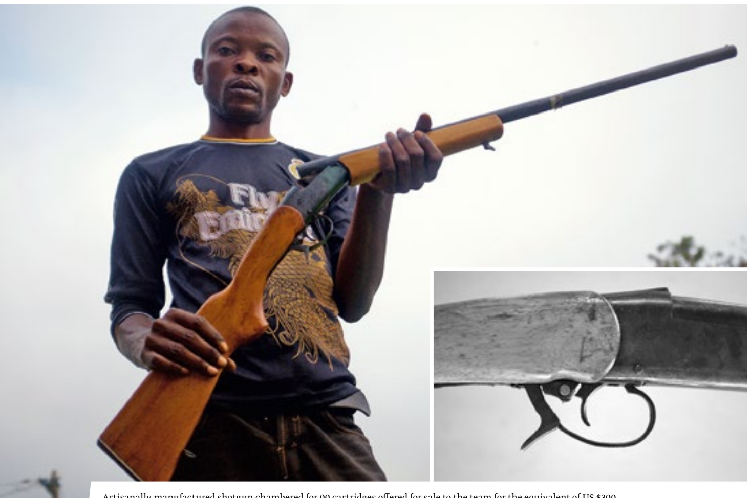
Artisanally manufactured shotgun chambered for 00 cartridges offered for sale to the team for the equivalent of US $300. The shotgun was fitted with a mechanical safety device to block the trigger mechanism (right).
