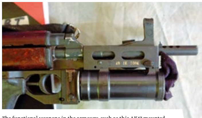
The functional weapons in the armoury, such as this AK47 mounted with an under-barrel 40mm grenade launcher, were serviced and oiled on a regular basis.
