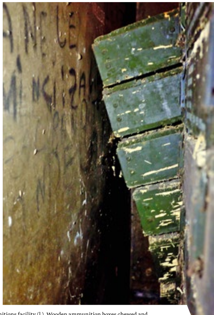
Highly flammable explosive resin on the floor of a storage site in Bokala munitions facility (l.). Wooden ammunition boxes chewed and weakened by termites (r.).
