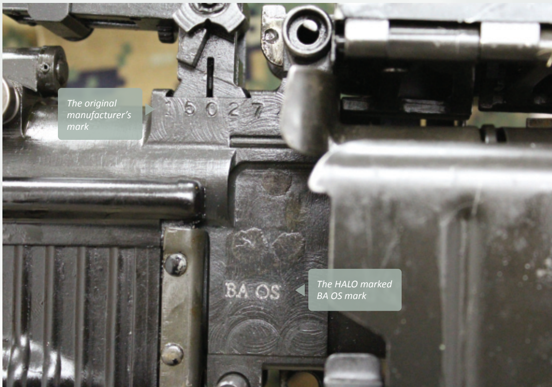
Figure 4. Close up markings on M60, Tuzla, February 2020; © The HALO Trust
