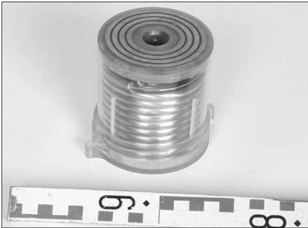
Figure 5: Cutaway model of a Stinger battery coolant unit
