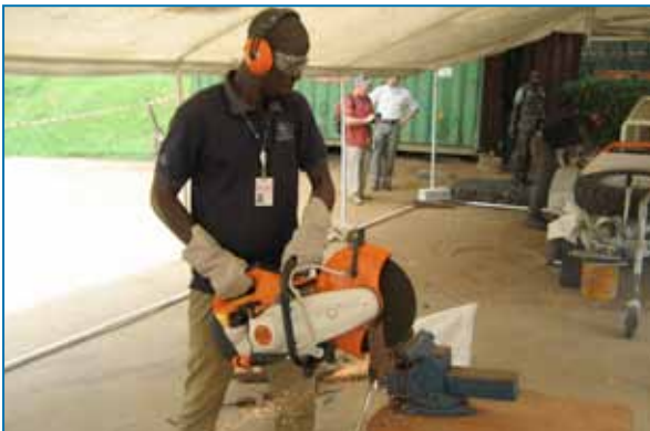
Mobile petrol chop saw. Source: HALO Trust.
