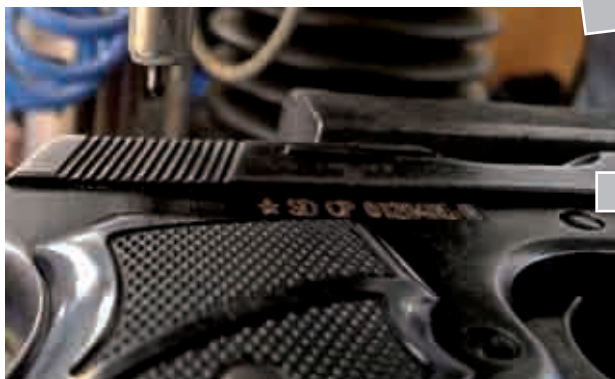
Marking: Dot-peen machines punch a set of marks onto the receiver or frame of a weapon to create letters, numbers and images giving each weapon a unique ID.
